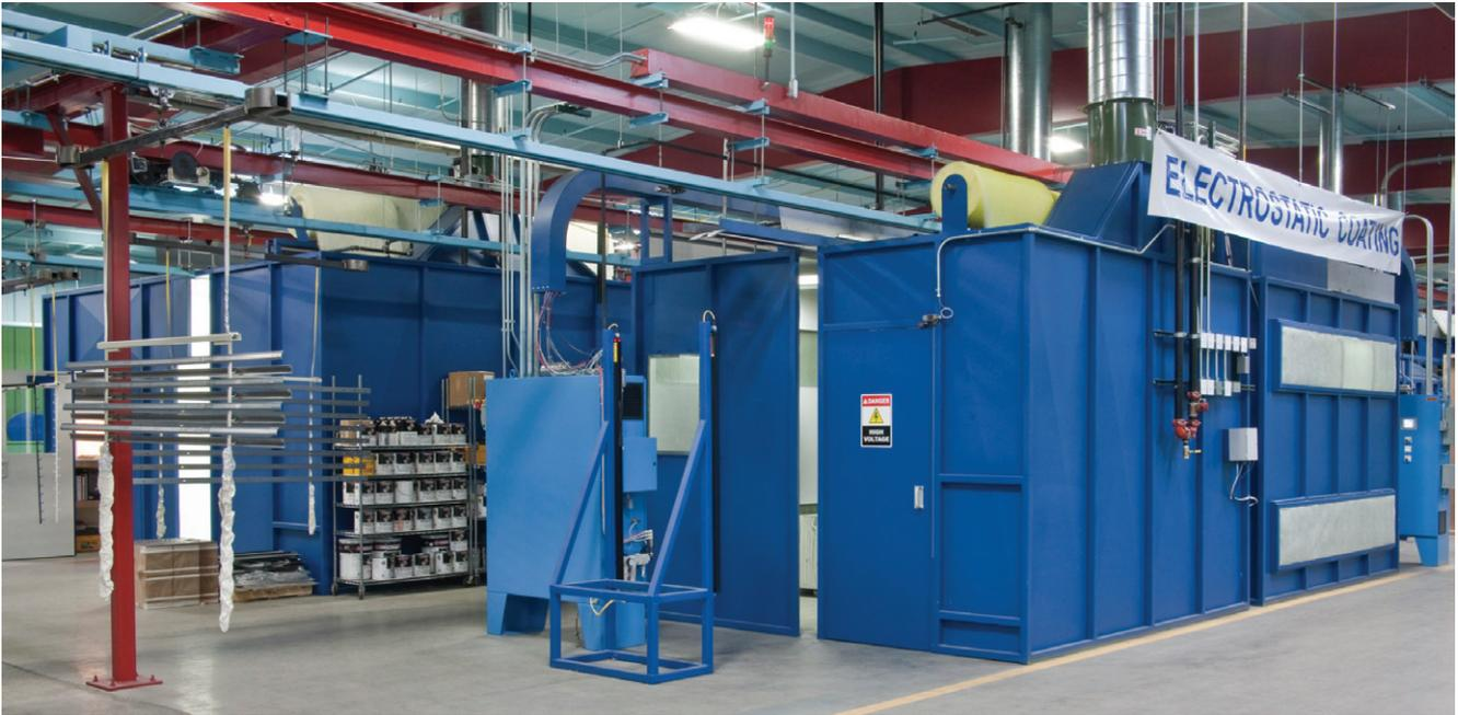
*Total Door's manufacturing floor with a UV coating and curing system.*
